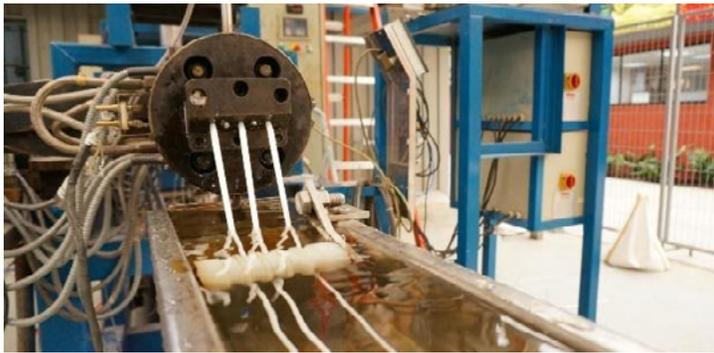
▲ MFC-reinforced PP extrusion
